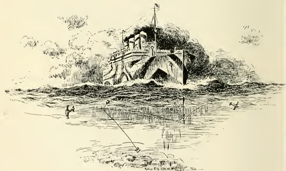
BURNEY GEAR. SKETCH SHOWING METHOD OF FITTING TO STEM OF VESSEL AND ACTION IN DEFLECTING ANCHORED MINE
