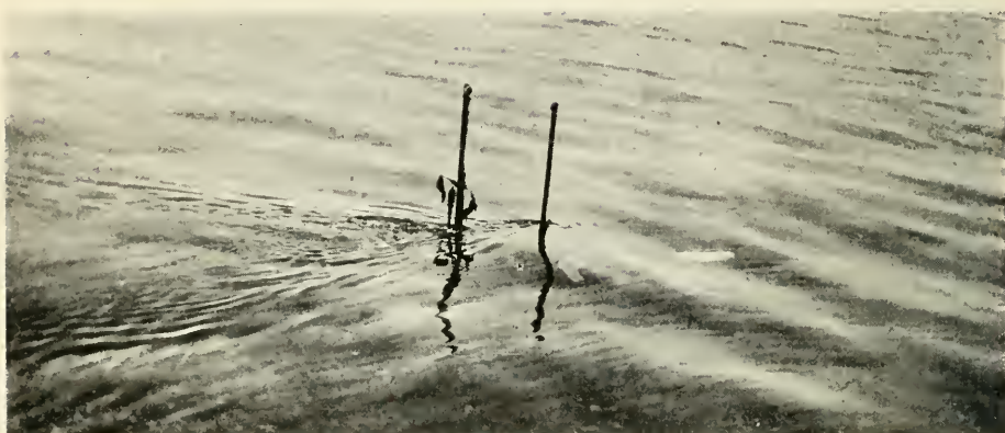
E-2 MAKING A PERISCOPE OBSERVATION AT SLOW SPEED. WHITE SPOT IN FRONT OF PERISCOPE IS SEA PLANE RECOGNITION MARK
