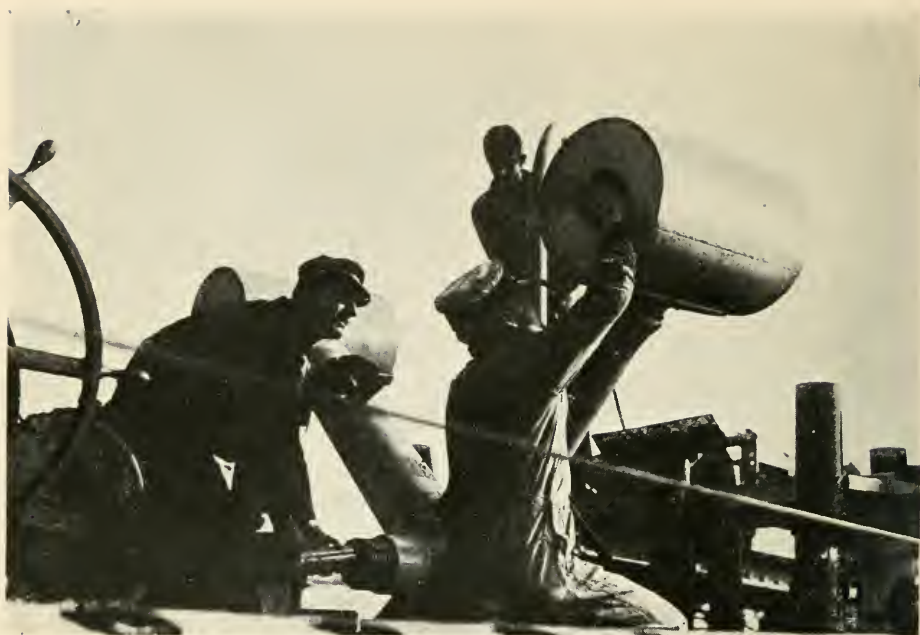
ADJUSTING TIMING MECHANISM ON DEPTH BOMB JUST BEFORE FIRING "Y" GUN
